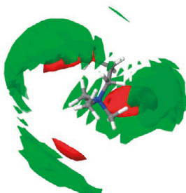
Fig. 4 c): Spatial density function (SDF) of the 20% probability surface showing the solvation of the molecule types around each other in 3D. Distribution centered around choline ChCl:LTA:W, the green isosurfaces correspond to L-tartaric acid molecules and the red to chloride anions.
