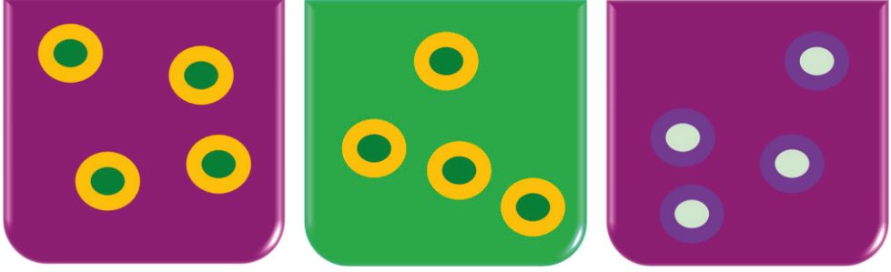
Figure 11: The effect of contrast variation on distinguishable structures in a neutron scattering experiment.
