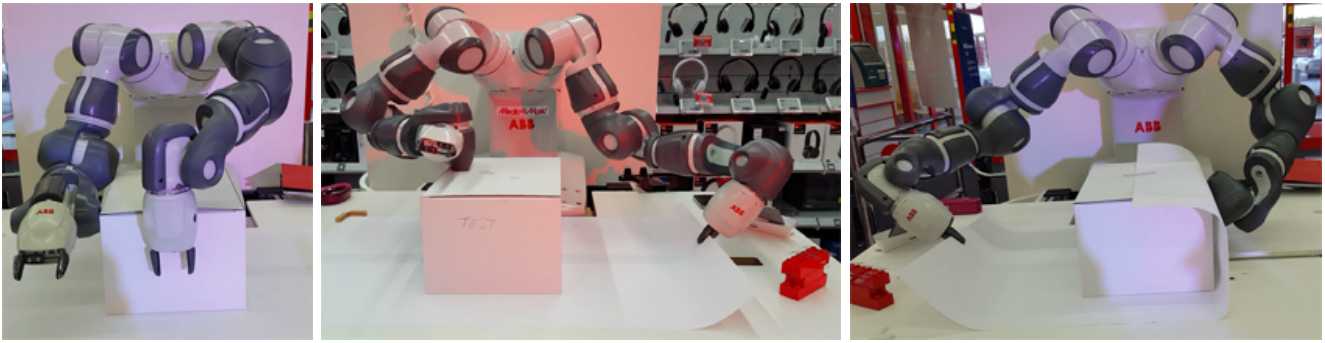
Fig. 2. L: The robot uses multiple contact points along the lower arms and the tool to push the box into its initial position; C: The table has an incision to let the robot fingers grip the paper without creasing it; R: One hand fixates the box while the other one folds and tapes the side.
