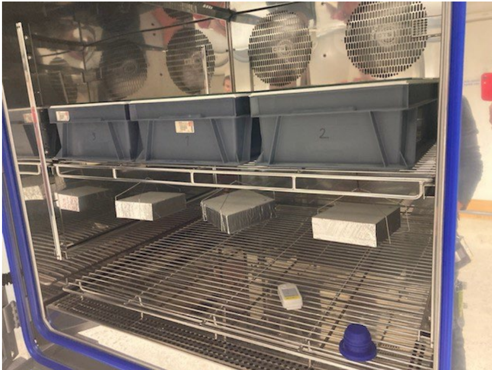
Figure 19: Three samples right before an MBV test. The samples are hanging in balances placed in plastic containers.
