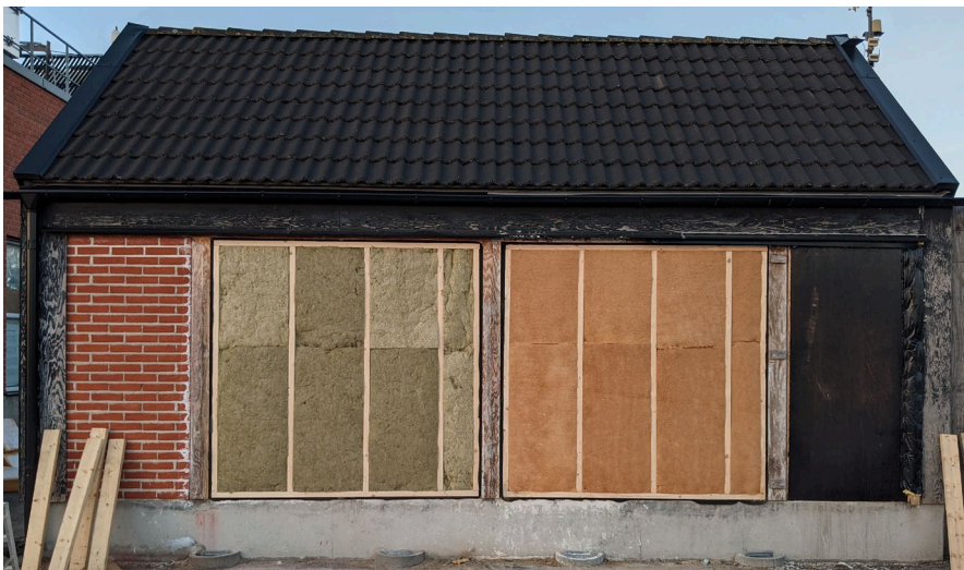
Figure 23: Southern facade of the test house. This photograph was taken while walls were being mounted to the house. The two timber framed walls are the ones tested. The brick wall is used in another project, and the wall to the right is just a 'dummy'.
