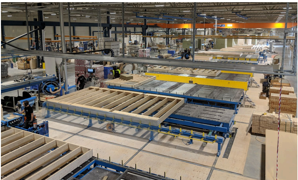
Figure 10: The floor assembly line from Lindbäck's factory in Piteå, Sweden. This is one of the companies within the reference group with a high degree of prefabrication. The photograph was taken in February 2019.
