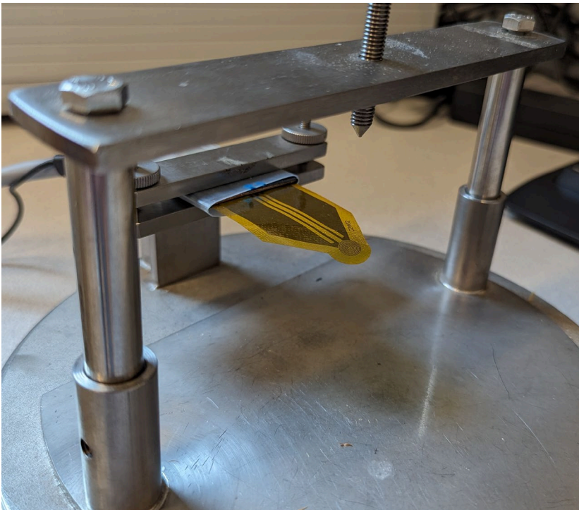
Figure 18: Holder for specimens and a sensor for TPS (HotDisk) measurements.
