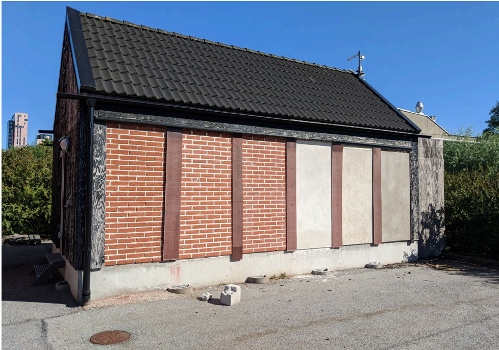
Figure 22: This photograph was taken of Lund University's facade laboratory in September 2020, before renovations were done within this thesis work. The building's normal use is to test the facade materials; at the time of the photograph, experiments were conducted with salt intrusion into brick walls.
