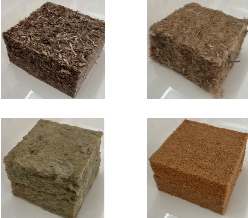
Figure 35: Samples of the insulation materials investigated in this paper. Clockwise, starting in the top left corner: eelgrass, grass, wood fibre, and stone wool (reference material).
