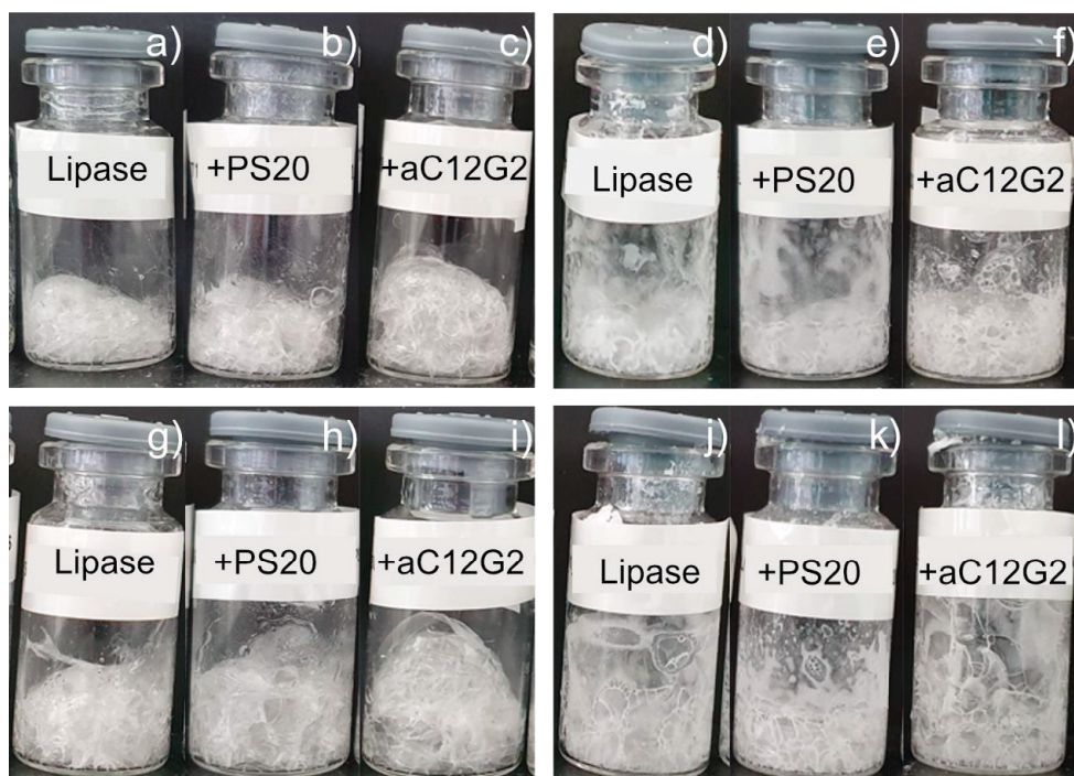
Figure 13. Representative images of vacuum foam-dried formulations in vials of 1/99 (% w/w) lipase/sucrose (a-c), 1/99 (% w/w) lipase/trehalose (d-f), 4/96 (% w/w) lipase/sucrose (g-i) and 4/96 (% w/w) lipase/trehalose (j-l), respectively (modified after Paper II ).
