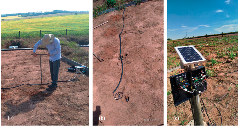
Figure 3.7: Photographs during drilling the soil (a) to install sensors at different depths (b), and a monitoring center station for soil water content (c).
