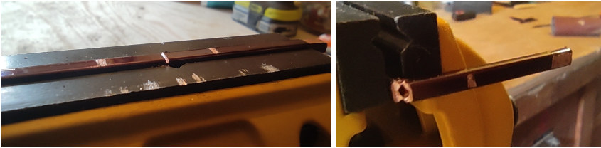
Figure 3.24: One of test samples 4-6 after being sawed (left) and after being bent (right).
