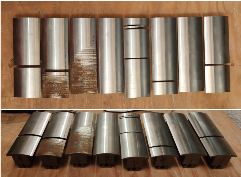
Figure 5.17: Broken rotor teeth before remounting. All pieces are marked and kept in the right order and direction.
