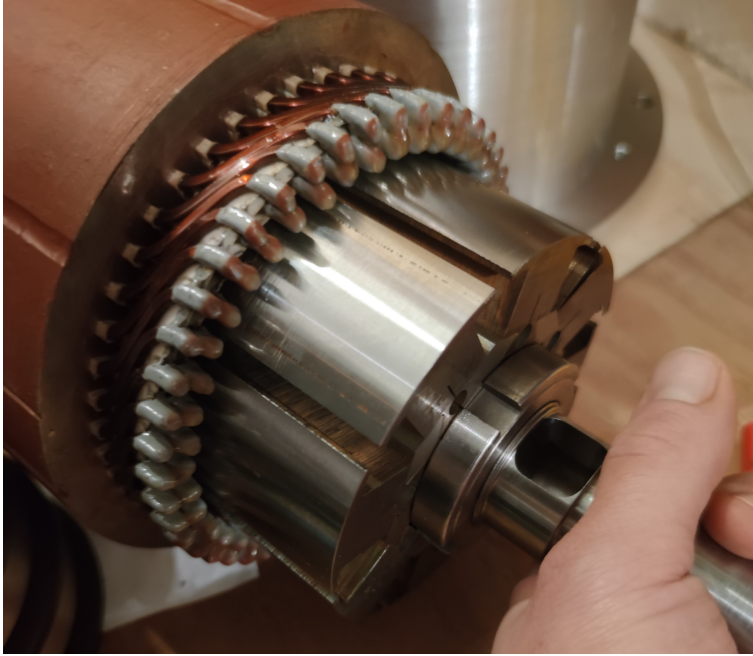
Figure 5.16: Grinded rotor inside stator.
