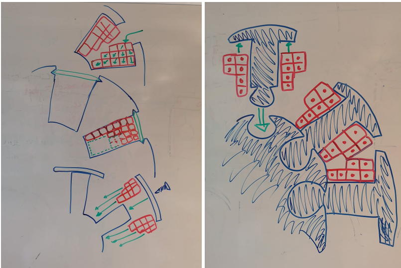
Figure 3.6: Early design sketches of rotor design options 1-3 to the left and option 4 to the right.
