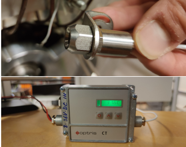
Figure 6.11: Photos of the optical temperature sensor with the sensor in the top photo and the electronic box in the bottom photo.
