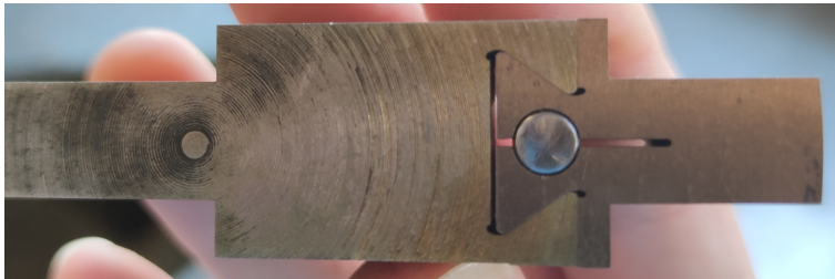
Figure 4.13: Photo of the tensile test sample with the final design and material choice.
