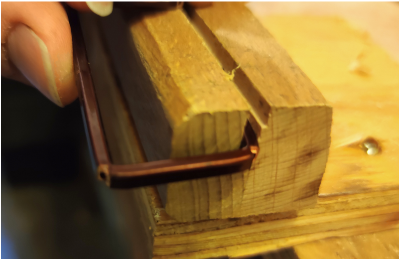
Figure 3.27: The rig for folding the coils, with a conductor with the first end turn completed.
