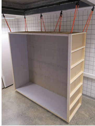
Figure 5. Photograph of the measurement setup used for the upper room structure.
