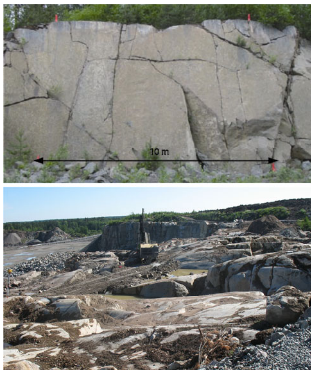
Fig. 2 Top quarry face at Olunda, bottom surface at Olunda after removal of the overburden
