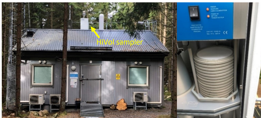
Figure 6 Left: The DHA-80 sampler on the roof of the Hyltemossa site. Right: Interior of the DHA-80 sampler, showing the filters mounted on filter holders.
