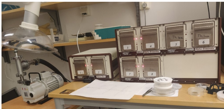
Figure 8 The alpha detector setup used for measurement of the membrane filters.
