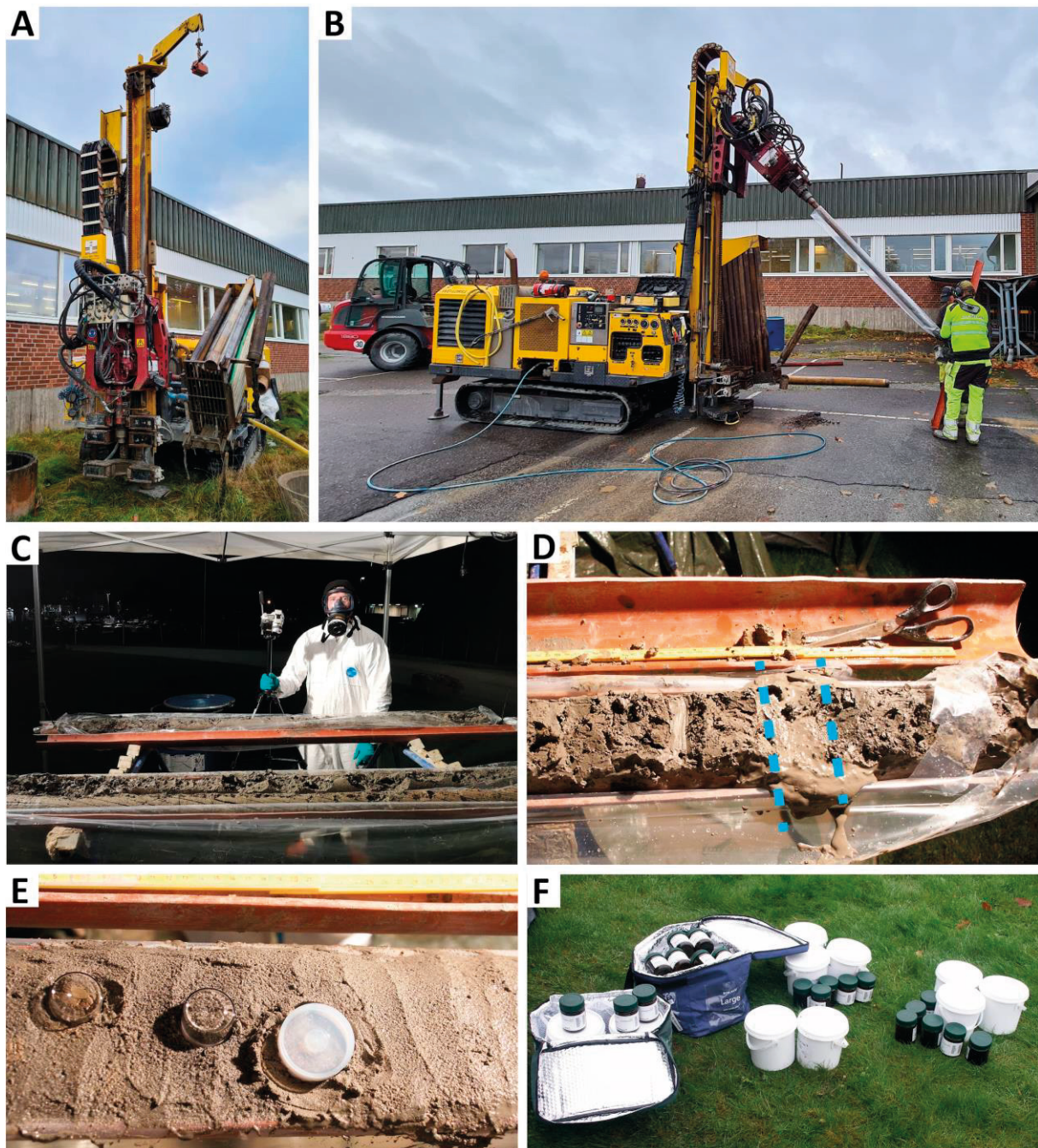
Figure 13. Photographs from the Alingsås laundry site during a fieldwork campaign in October 2020, illustrating A) a sonic drilling rig in operation, and B) the extraction of a drill core. C) displays parts of the outdoor fieldwork laboratory with core sections mounted on a rack for logging and sampling. D) highlights a transmissive fracture in an otherwise tight, clayey silt segment of one of the cores. E) shows the process of sampling in a well-sorted sandy segment within a core, and F) shows a collection of samples gathered for chemical and grain size analysis prior to shipment to the laboratory.
