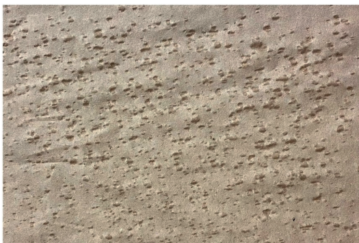
Fig. 13. Wet dots on a paper sheet exposed to water spray for 1–2 s.
