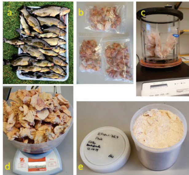
Figure 4 Sample preparation for fish samples prior to gamma spectrometry analysis. a) Tench ( Tinca tinca ) prior to filleting. b) Fillets cut to smaller pieces. c) Freeze-drying in zip-lock bags. d) Freeze-dried pieces of fish fillets. e) Powdered freeze-dried fish meat in 200 ml beaker.
