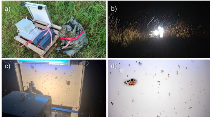
Fig. 1.6: Operation of a machine vision-equipped moth light trap [53]. a) Weather-resistant system with UV light ring, camera, and white sheet. b) Operated at night for optimal moth attraction. c) Attractions of many moths, demonstrating effectiveness. d) Captured high-resolution image.
