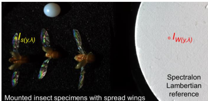
Fig. 4.7: Hyperspectral scan scenario where the sample and reference are placed on the same plane. This configuration ensures close pixel-by-pixel matching between the camera's Y pixels and the reference.
