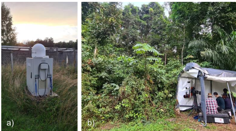
Fig. 1.7: Examples of radar and lidar in field research. a) Radar at Stensoffa field station in Sweden generates data on bird migration patterns. b) Lidar in the Tai virgin rainforest, Ivory Coast, provides insights into insect behavior and populations.
