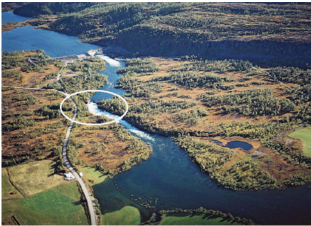
Fig. 1 Aerial photograph of the location of the embankment test facility in Røssåga river. In the upper left part is the Røssvatn reservoir impounded by the Røssvassdammen dam (from Høeg et al. 2004)
