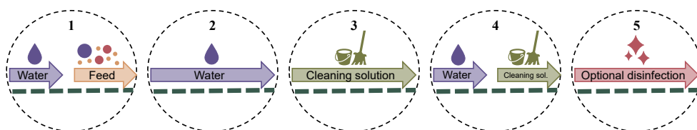
Figure 8: Schematic showing the steps of a membrane cleaning cycle.
