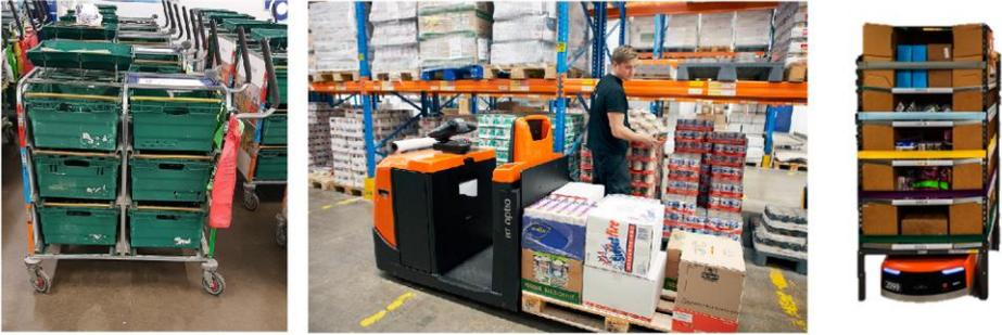
**Figure 5:** Examples of vehicles used in warehouses. On the left is a trolley with 6 bins where each bin can be used to collect an order using sort-while-pick batching [19]. In the middle is a forklift carrying a pallet on which a set of products or orders is placed, e.g., using *pick-and-sort* batching [20]. On the right is a vehicle carrying a pod (a movable rack) [21], deployed in a Robotic Mobile Fulfillment Centre (a type of *parts-to-picker* warehouse) [6].
