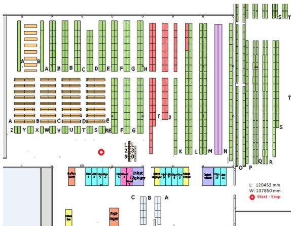
**Figure 4:** Top-view of the Aba Skol AB warehouse. The picking zones are color-coded. The red circle denotes the most commonly used depot location.
