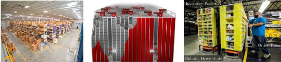
**Figure 2:** The insides of warehouses can look very different. On the left is an example of a picker-to-parts warehouse with a conventional layout [7]. In the middle is an RCSR system and on the right an RMFS [6]. The pickers in the latter two cases are only involved with sorting, packing and checking products.
