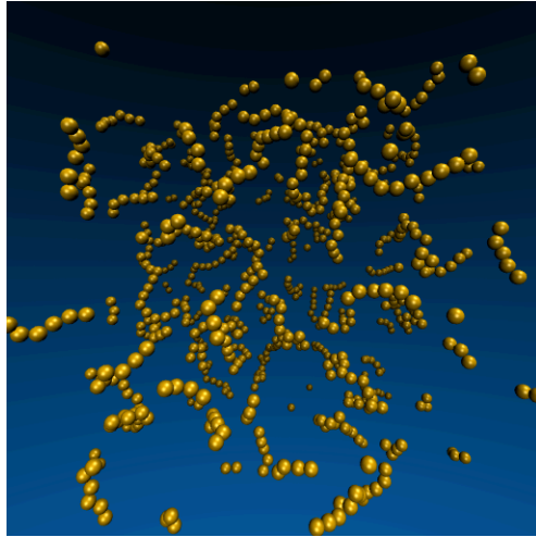
Figure 7.6: Simulation snapshots of structures obtained at low volume fractions (1%). in systems in which the grafted particles also carry a weak charge, in solutions containing 0.01 mM monovalent salt.
