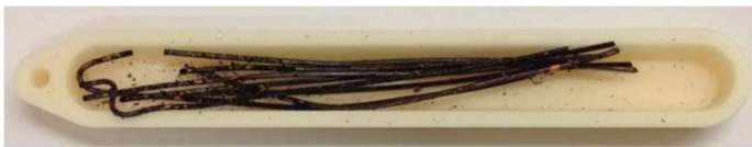
Fig. 7.1 Picture of the enameled wires after thermal stress of 275°C for 168 hours seated in the alumina boat crucible
