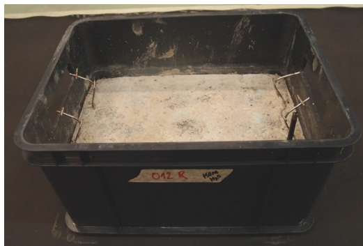
Fig. 1. Example of the concrete slab in the plastic mold. The welded reinforcement bar can be seen in the bottom right corner. On both left and right edges the edge of the stainless-steel mesh is visible.
