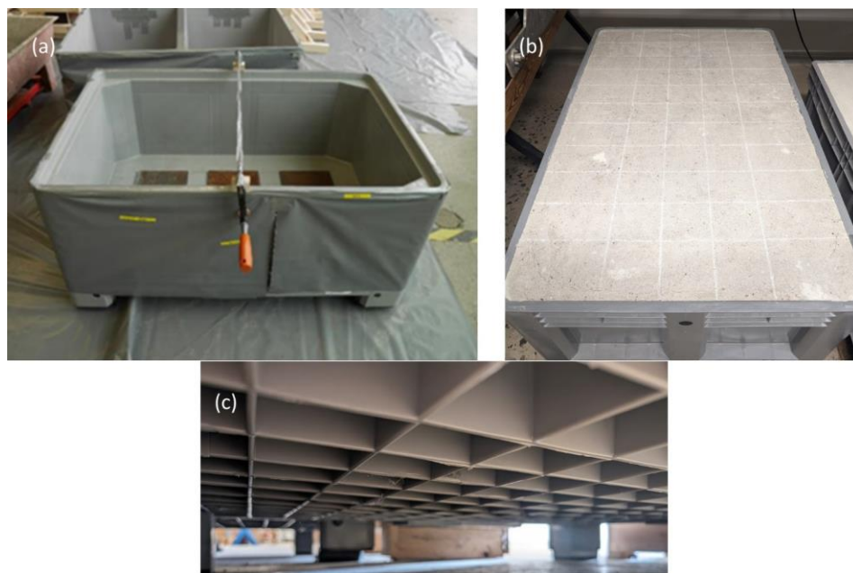
Figure 35. Concrete slab specimen. (a) Heavy-duty plastic container before casting. (b) Slab after curing and surface removal. (c) Reinforced bottom showing no signs of buckling. Figure from (Nilsson et al., 2024b).
