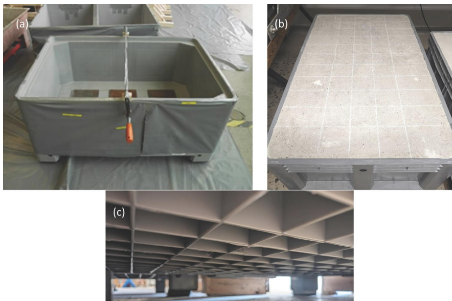
Figure 2. (a) Plastic container used as a mould for the concrete specimen. (b) Specimen after 5 years. (c) Reinforced bottom shows no indication of buckling.
