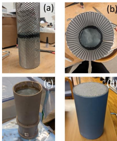
Figure 28. Cylindrical specimens. (a – b) Steel mesh and centred plate. (c) Specimen after casting. (d) Specimen after curing. Figure from (Nilsson et al., 2024a).
