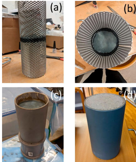
Fig. 5 (a) and (b) The plate discs were attached to cylinders of expanded metal (steel) before casting. The discs were adhered using silicone. (c) The cylinders were cast at full length (250 mm) and cured. (d) After being cured for 5 weeks the cylinders were cut to 200 mm by removing 25 mm from both ends of the concrete cylinders.
