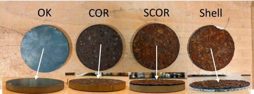
Fig. 3 The plate discs that were embedded in concrete. From left to right: OK (non-corroded), COR (uniform corrosion); SCOR (uniform corrosion with a layer of shell-type corrosion product glued on top); Shell (only shell-type corrosion product).
