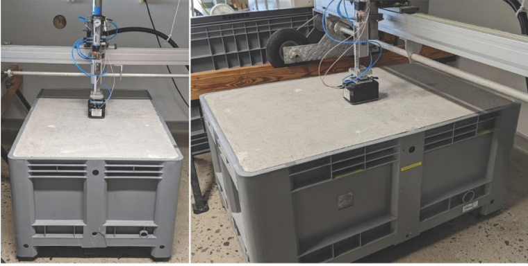
Figure 8. The concrete slab specimen and the xy-scanner used to control the ACS M2502 fixed dual aperture array.
