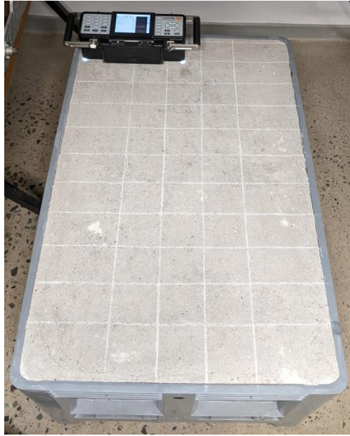
Figure 44. Measurement grid for the MIRA.
