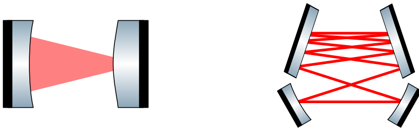
Figure 3.15: Examples for power scaling, with a concave-convex setup (left) and beam folding (right).
