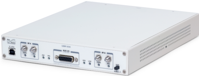
Figure 3.1: The NI-USRP 2953R 40 MHz. Also known as Ettus X310 with two CBX40 daughterboards.
