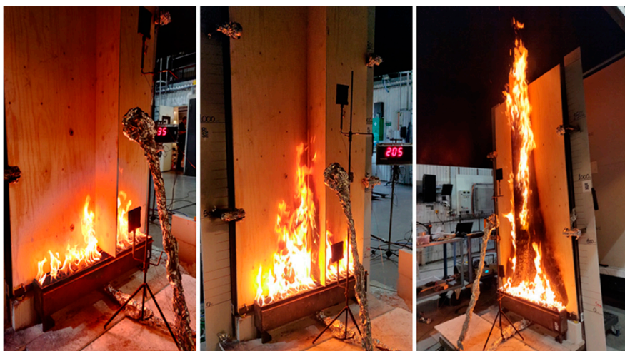
Figure 11. Intermediate-scale test setup for plywood façade with added central wing flange.
