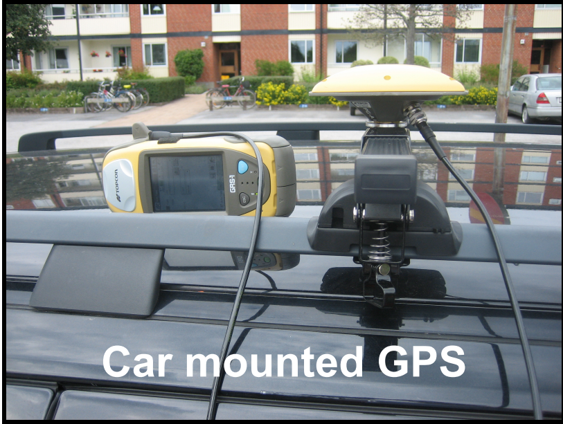
Figure 2.6: High accuracy GPS with an external antenna mounted on the top of the car.
