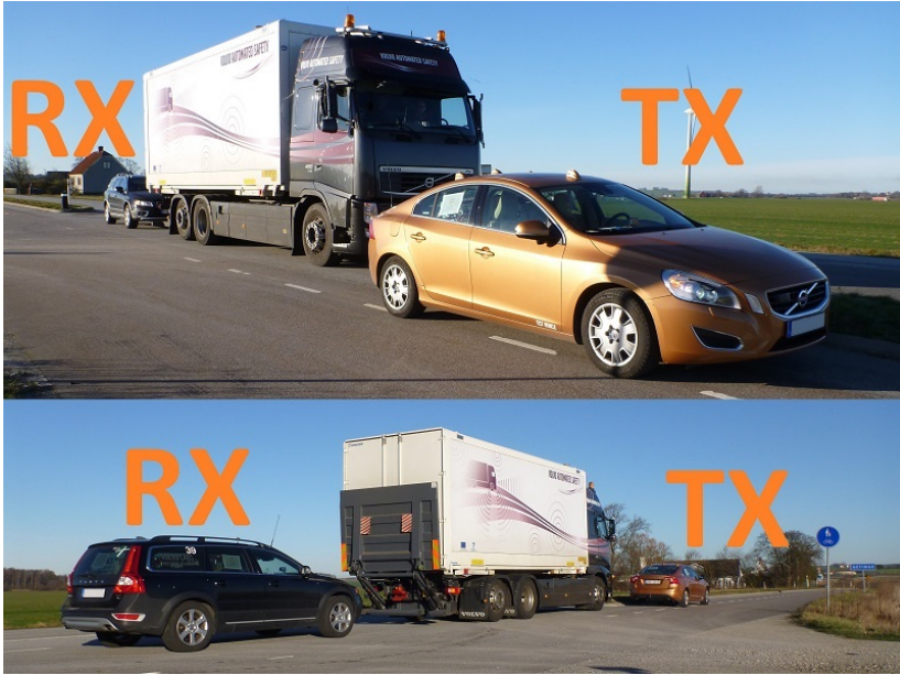
Figure 3.1: The two cars at TX/RX and the truck as obstacle used in the measurements. The total truck length was 9.8 m with a container width of 2.6 m and height of 4.0 m from the ground.
