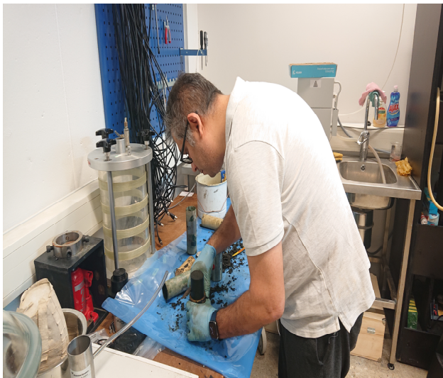
Figure 9: Trimming samples to reach dimensions (50mm diameter and 100 mm height) for FFR, and UCS test (photo by Torleif Dahlin)
