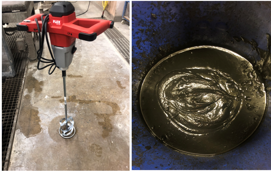
Figure 5: Left: Electrical paddle mortar mixer, right: Dredged sediment (Photo by author).
