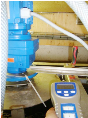
Figure 1 Torque measurement device for determining the mixing intensity in the coagulation and flocculation tanks.
