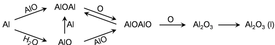
Figure 2.3: Dominant reaction pathways for the gaseous aluminum-steam reaction system. Figure reproduced from ref. [56].
