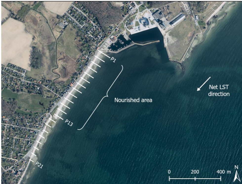
Figure 5.1: Map showing the study site and the location of the survey transects P1-P21. The nourishment is placed between the harbour mole and the terminal groin covering transects P1-P13.
