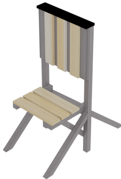
Figure 1: Experimental setup with horizontal boards (decking) and south-oriented vertical boards (cladding).
