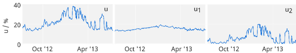
Figure 2: The moisture content, u , decomposed into a sheltered part, u_1 , and a rain-induced part, u_2 .
