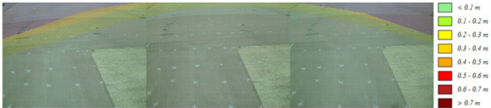
Figure 6. Example of camera accuracy output following calibration using T-Calibration software (T-Analyst, 2019)
