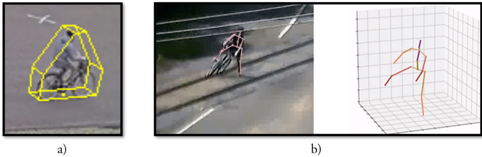
Figure 13. Examples of trajectory representation: a) The central position of the road within the 2D projection on the ground plane, as defined by the bounding box (T-Analyst, 2019), b) sequence of reconstructed 3D poses derived from corresponding 2D keypoints
