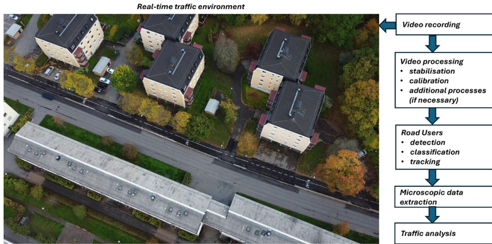
Figure 1. Schematic diagram illustrating the sequential stages of transforming video data into advanced traffic analysis
