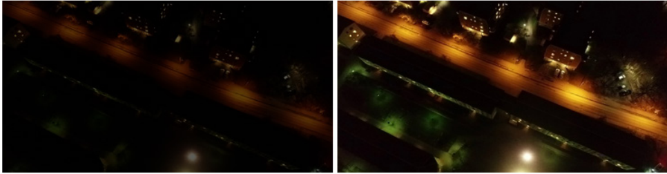
Figure 7. An example of brightness adjustment for the same camera view (before adjustment—left; after adjustment—right)
