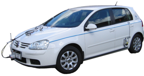
Fig. 3. The vehicle testbed used in the experiments. The velocity sensor is placed at the front end, aligned with the longitudinal axis. The roll and pitch angle sensors are situated at the front end and in front of the rear wheels. The vehicle was also equipped with a GPS receiver during the experiments.
