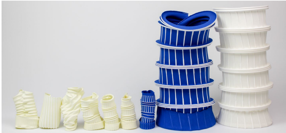
Figure 11. The first tower prototype, inspired by a rib cage, emerged from an iterative design process, showing behaviors of bending, arching, and rolling. This prototype stands compressed, can be stretched and elongated, and confirmed the self-supporting structure theory by maintaining its shape and position for months on display and landing upright when dropped from 1.5 meters. Dimensions: Ø200 mm, height 450 mm.
