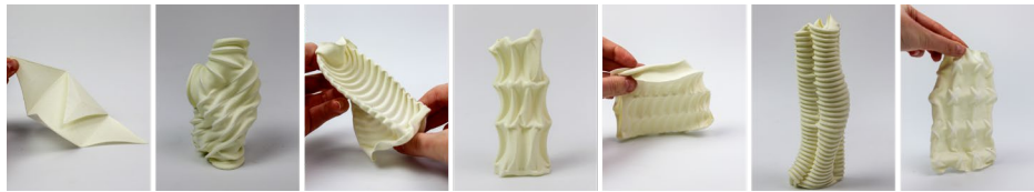
Figure 4. Small-scale probes designed to test geometries for structural behavior across controlled textile and filament variables.
