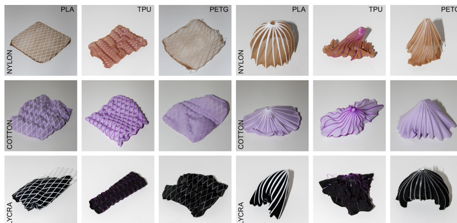
Figure 3. Matrix of initial experiments testing warping behavior across variables of filament, textile and geometry type.
