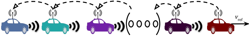
Figure 3.5 A vehicle formation implementing a serial consensus controller. Each vehicle measures the relative distance and velocity to the predecesing vehicle and signals the perceived relative distance to its follower.
