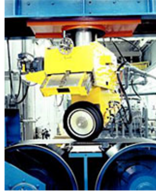
Figure 4.5: Tyre test rig at Calspan Tire Research Facility, image from calspan.com.
