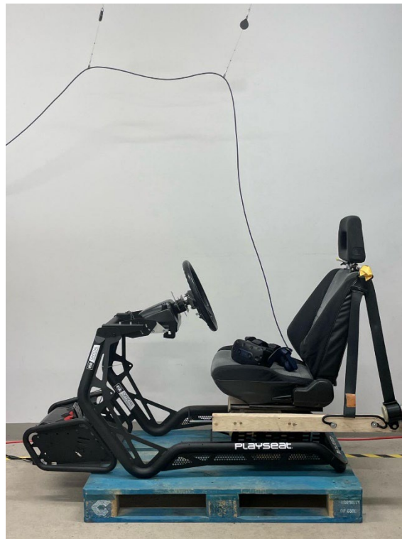
Figure 47. The VR setup adopted in the driving behavior in smoke experiments.
