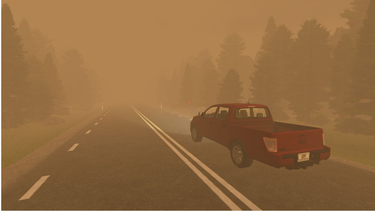
Figure 48. Road and the vehicle controlled by the participant. In this figure, the extinction factor K equals to 0.05 \text{ m}^{-1} .
