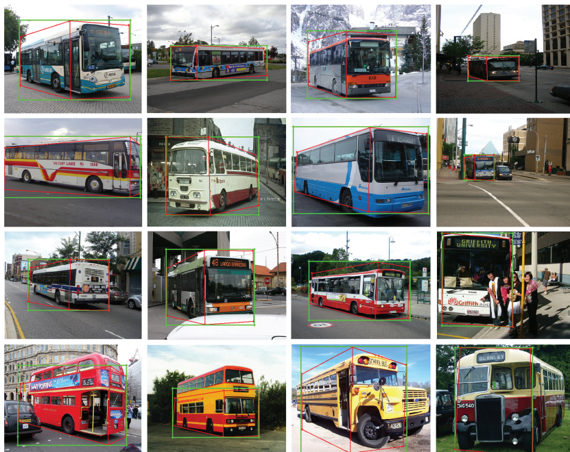
Fig. 7. Example results. Detected bounding boxes are shown in green and their layout in red. The first three rows shows correctly detected objects with roughly correct pose. The method was able to automatically handle cases when only one side is visible. The last row shows the buses of which the pose estimation is less accurate.
