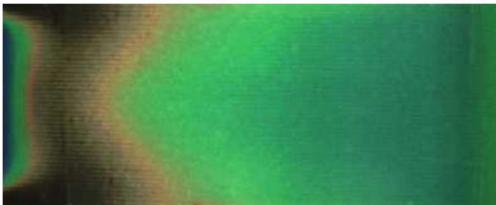
Figure 4: A typical LCT image behind a single bluff body where \dot{q}_w = 1850 \text{ W/m}^2 and \text{Re}=100,000 .
