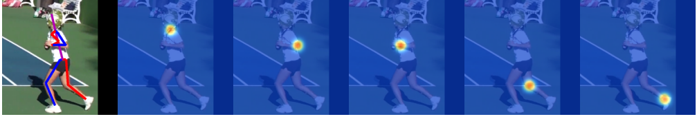
Figure 3.9: Heatmap-based 2D pose estimation. The model predicts one heatmap per joint (right). The final pose is given by the maximum activation for each heatmap (left). Image from [80].
