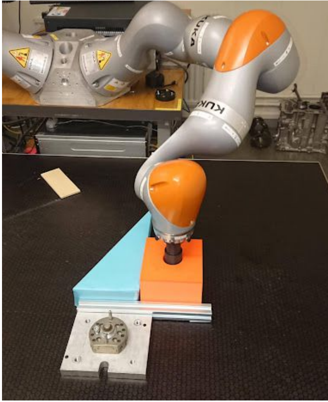
Figure 12: Experimental setup for the peg-in-hole task, where a peg (black) is inserted into a box (orange) with a hole.
