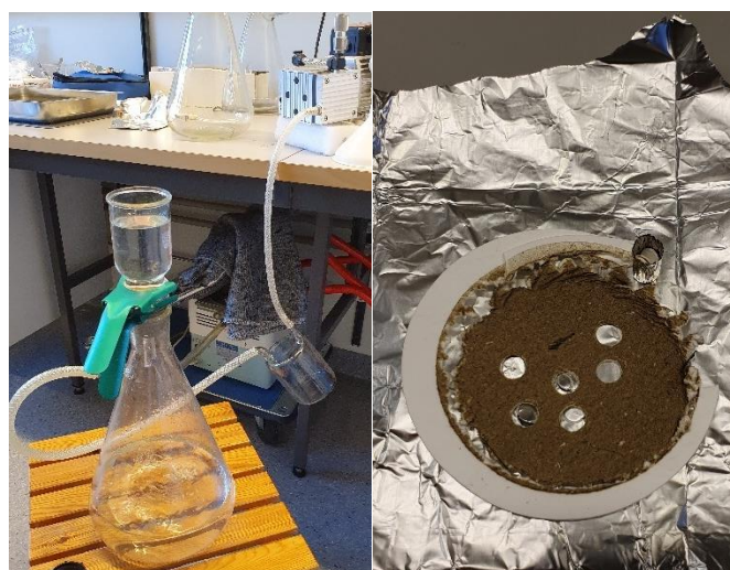
Figure 12 Left: Apparatus for vacuum filtering of seawater samples. Right: Filter with after filtration. The punched smaller pieces are taken further to ^{14}\text{C} analysis.
