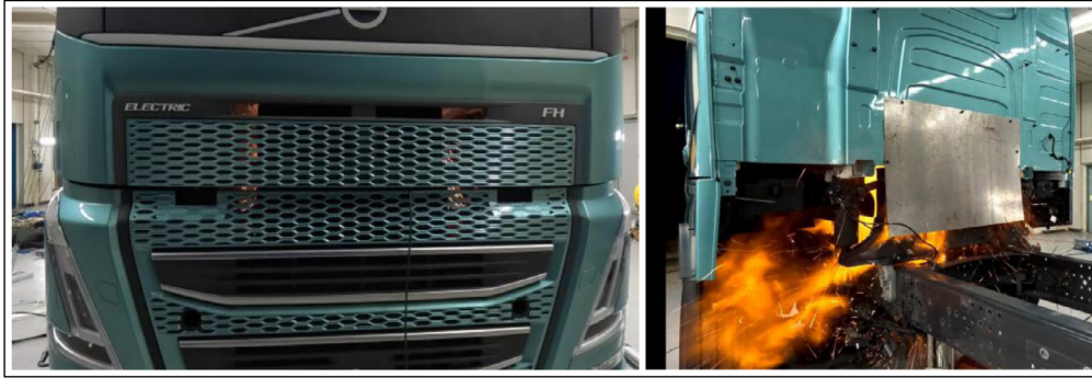
Figure 6 Frames with explosion extracted from film with 13 g released H_2 .
