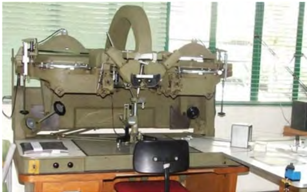
Figure 6.6. The Wild B8-S stereo-aviograph in the “Phototeket” annex.
