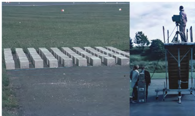
Figure 8.36. The test set up of a model city at the Bulltofta airfield in 1969 for developing and applying infrared photographic technology in micro- and local climatological research. (Photo J. Åkerman -69)
