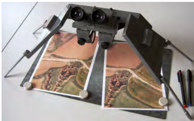
Figure 6.3. Standard student stereoscope for air photo interpretation. (Photo J. Åkerman 2020)
