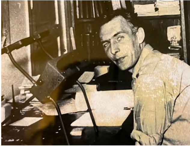
Figure 6.4. An early type of stereoscope for air photo interpretation was used by amanuensis Harald Svensson in 1955. ( Photo probably by G. Rasmusson -55 )
