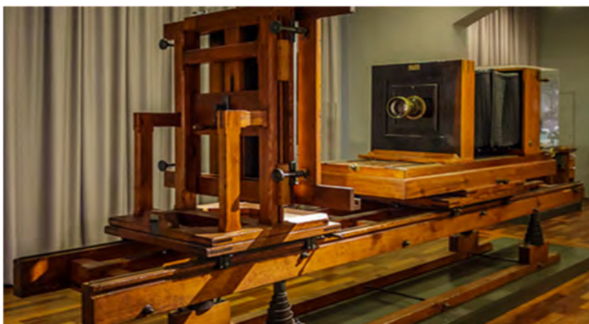
Figure 6.7. The large-scale reproduction camera in the Geographical photographic laboratory. (Photo by J. Åkerman 1969)
