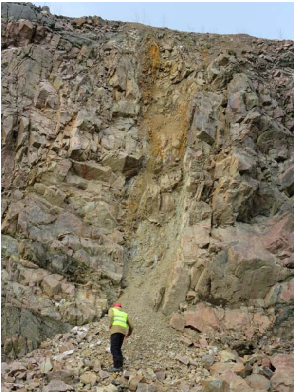
Figure 1. Example of a vertical weathered zone in the quarry which is situated next to the survey area. Notice the highly fractured character of the rock mass surrounding the zone, it is typical for the rock that is exposed in the quarry.
