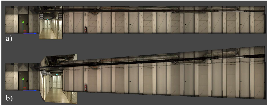
Figure 22 – Illustration of the differences in the projections used for the scenarios. This is not the participants' view. The camera is located on the far left indicated by the green arrow. a) Side view of a corridor scenario using default projection. b) Side view of a corridor scenario using the vertex displaced projection using a _FarScale of 2.0 at a _NormalizingDistance of 25 meters
