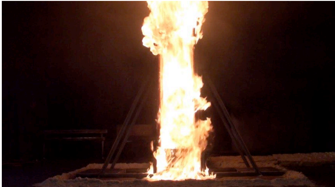
Figure 7: The whole area of the material plates is burning together with the melted material on the floor.
