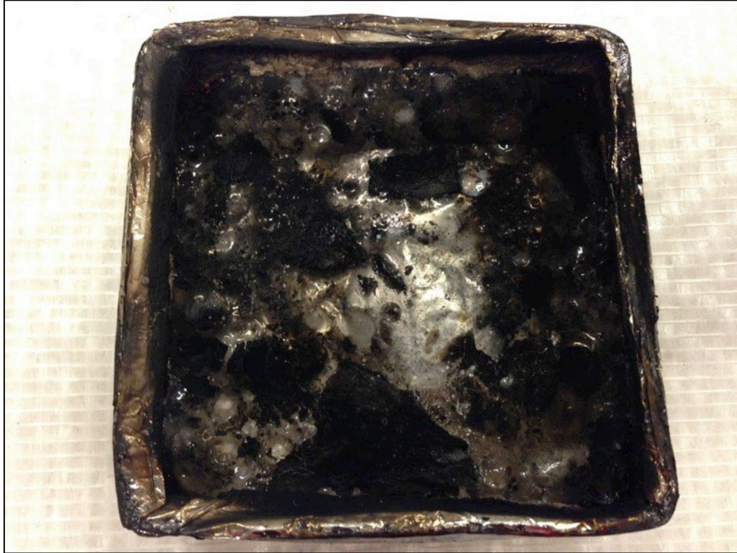
Figure 2: Colourless glass-like residue after combusting borated polyethylene.
