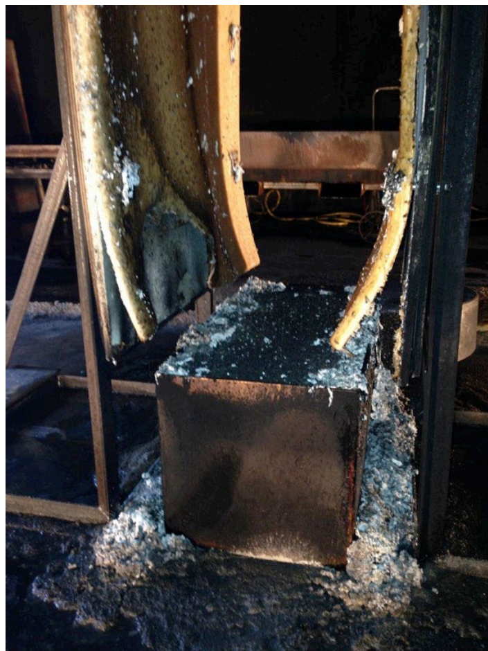
Figure 10: The melted material is piled up beneath the material plates.
