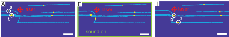
Figure 6.5: Frames of exemplary sorting application video. A (left) before activation of thermoacoustic streaming. The two particles a and b (marked with white circles) flow close to each other from left to right. E (middle) during trigger. Particle a moves from the side of the channel to the center, moving in a bow around particle b. I (right) after trigger ended. Particle b remained on its trajectory, as indicated by blue streamlines while particle a has moved and is now more centred in the channel.
