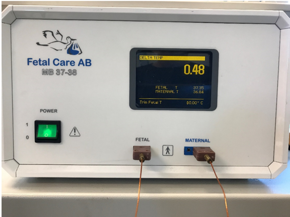
Figure 3 The Fetal Care Temperature monitor. Fetal and maternal temperatures are shown with two decimals. The delta temperature is also displayed (fetal minus maternal temperature).
