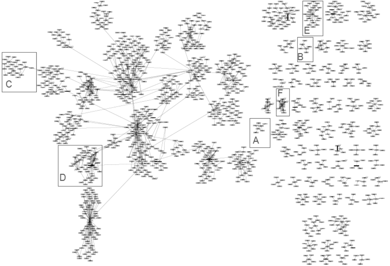
Figure 2. Explicit issue networks in the Android IMS. The figure shows all networks containing five or more issue reports, in total 1,382 reports and 2,060 links. A to F are the sample link clusters we analyzed qualitatively.
