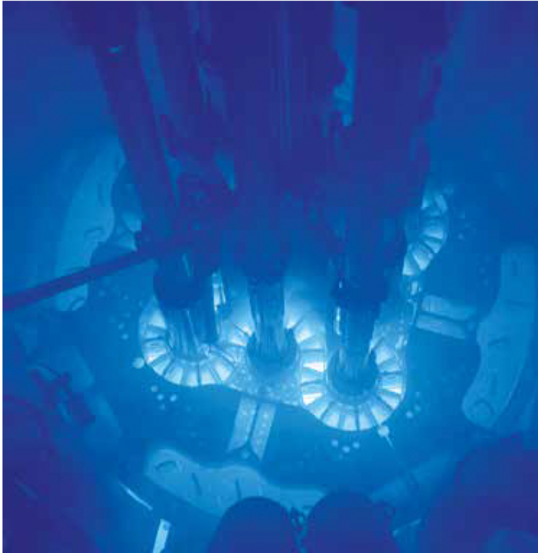
FIGURE 16 Cherenkov radiation surrounding the advanced test reactors core. Photo by the Idaho National Laboratory's ATR, 2009.
