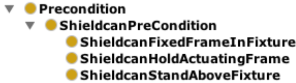
Figure 11: The device requirements of the skill ShieldCanInsertion are modelled in an ontology. The ManipulationRequirement which several skills inherit from, is that a gripper has to be mounted on the robot. The ShieldcanFixtureRequirement and the ShieldcanForceSensorRequirement list that there must exist a fixture and a force sensor that have to be vertically aligned (not shown in the picture).
