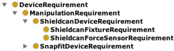
Figure 11: The device requirements of the skill ShieldCanInsertion are modelled in an ontology. The ManipulationRequirement which several skills inherit from, is that a gripper has to be mounted on the robot. The ShieldcanFixtureRequirement and the ShieldcanForceSensorRequirement list that there must exist a fixture and a force sensor that have to be vertically aligned (not shown in the picture).
