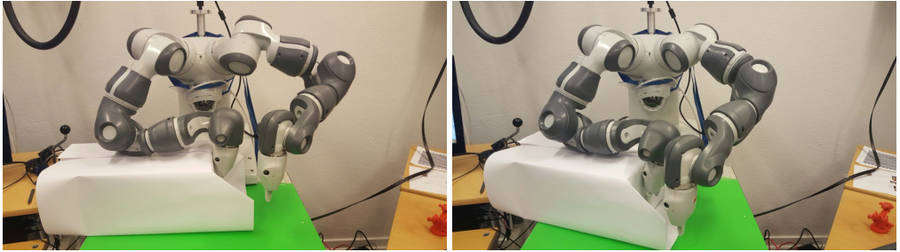
Figure 4: Paper folding (left). When rotating the box, only two positions must be updated (right).
