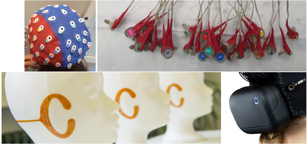
Figure 1.3: In the top, a Biomsei EEG cap (left) with corresponding EEG electrodes (right). The bottom left show cEEGrid arrays with electrode placement around ears (source: https://commons.wikimedia.org/wiki/File:CeeGRID.jpg ). The bottom right shows an battery driven amplifier for a mobile EEG cap.
